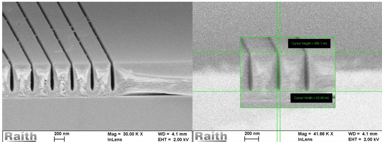
Figure 1: a, profile of the trenches written in SML550 resist viewed at an angle of 80°, b, Close up view of the trenches seen in the left also viewed at an angle of 80°.
