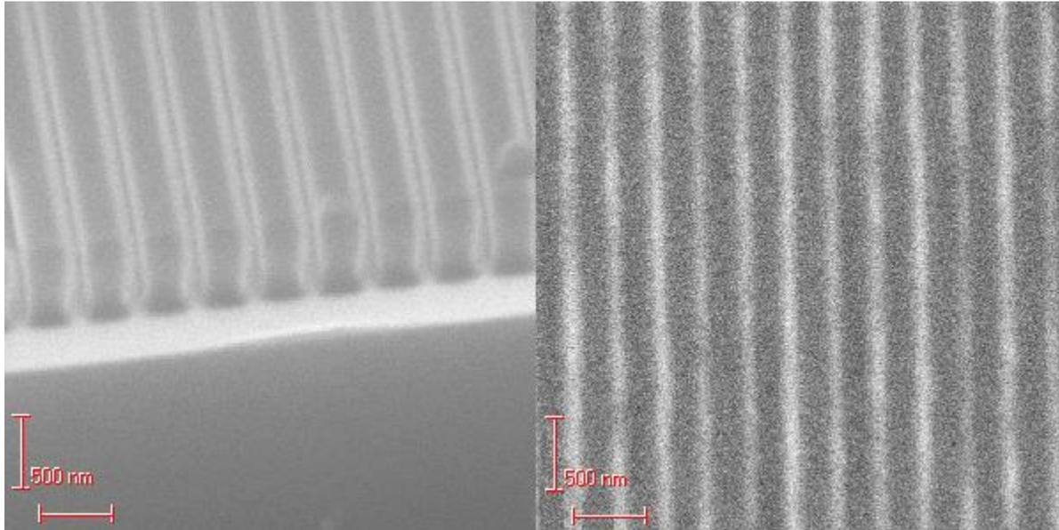
Figure 2: a, profile of the trenches written in SML550 resist viewed at an angle of 52°, b, Top view of the Aluminium lines.
