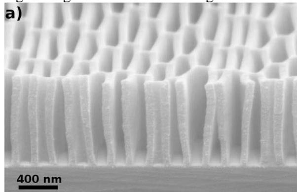
Figure 4: Scanning electron microscope (SEM) images of dense lines exposed in 1 $\mu$ m thick PMMA on Cr/Si substrate (tilt 70°) exposed at 100KV [3].
