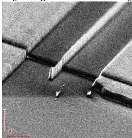
Figure 3: SEM image of a Schottky gate structure with an aspect ratio of 5.2:1.
